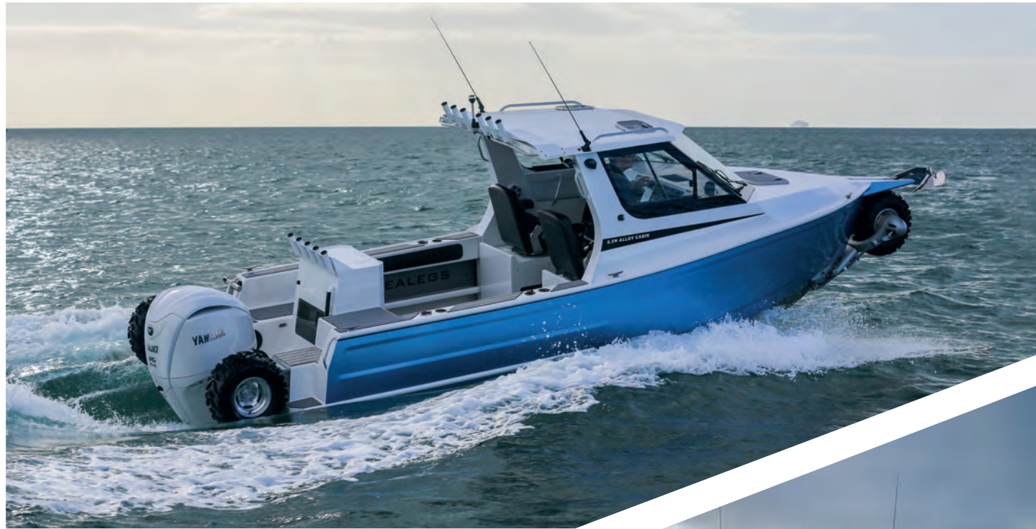
Above: The V6 Yamaha 300hp provided good acceleration. Right: Sealegs' amphibious system offers All Wheel Drive and diff-lock
